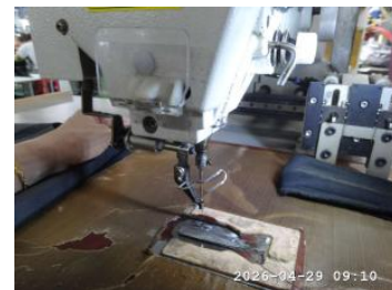
NC. Needle guard was placed in wrong position..jpg
